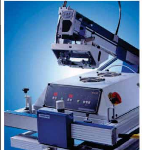
AN INTEGRATED FLASH reduces setup time by eliminating the need to walk around the machine to change flash times. Integrated flashes can be controlled from the master control panel.
