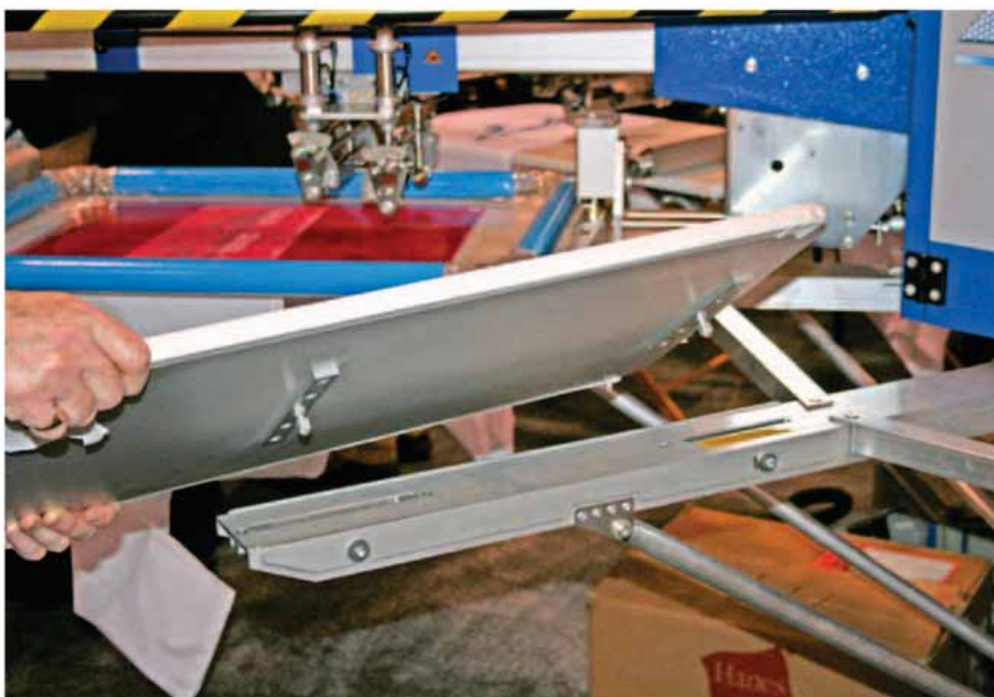
PRESSES VARY WIDELY in how many steps are involved in changing out pallets, which can greatly impact press setup times. Some machines allow you to touch an icon on the control panel, and the pallets unlock.
