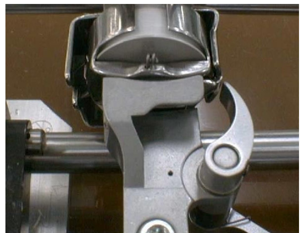
Chucking Device Opened (Bobbin case is released)
