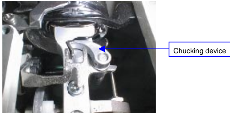
Bobbin Case - Chucked at the Machine Side
